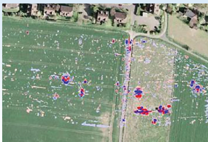
SQUID-GRADIOMETER MEASURING DATA , GEO-REFERENCED AND EMBEDDED IN AERIAL IMAGE BLUE - RED CONTRAST REPRESENTS MAGNETIC ANOMALY LIKE AIRCRAFT BOMBS AND FILLED CRATERS
